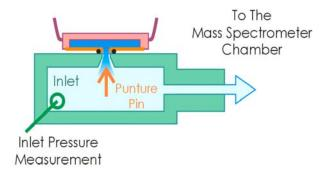
pin will be driven to pierce the package lid. This mounting procedure places most of the
