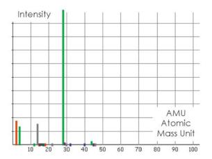
This raw data is corrected from the background effect to form the mass spectra of the gas sample (peak intensities for each detected AMU). The next step consists in associating these peaks with individual gases, taking into account the interfering spectral peaks and instrument sensitivity. The final quantitation is calculated in % or ppm by volume concentration.
