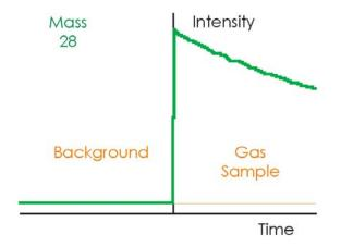
The analog signal generated is then digitized to form a raw data file.
